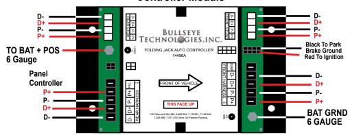
If a fuse is to be inserted between the Controller Module and the Positive Battery connection, a 60-amp fuses recommended
